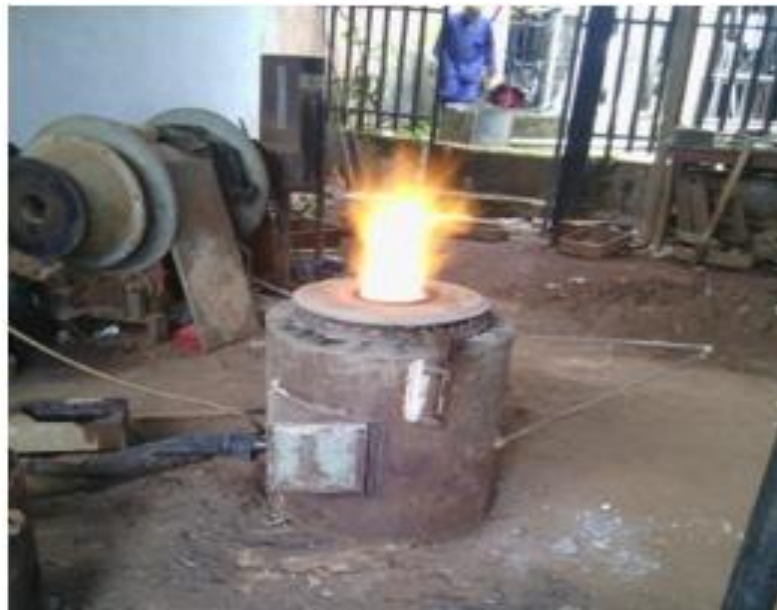
Fig 1: The produced oil fired crucible furnace
